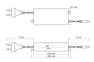
Fig.1. Dimension of power supply.
